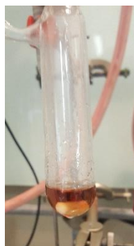
Figure 15 - Sample corresponding to Sample 1 in Table 10, after 1 hour (crude sample) with methanesulfonic acid.
